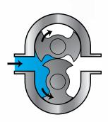
The pumping action of the rotary lobe pump principle is generated by the contra-rotation of two pumping elements (rotors) within a chamber (rotorcase).
