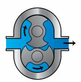
As the rotors pass the suction port, the cavity increases creating a pressure decrease, which induces the pumped medium to flow into the rotorcase.
